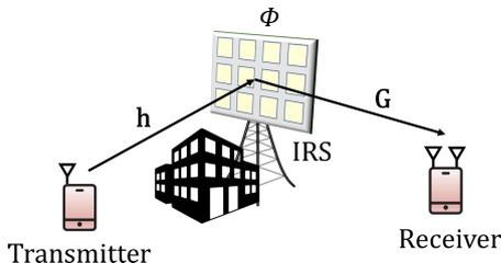
Fig. 1 System model of the proposed IRS-assisted STLC system.
